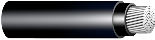
1- Core AL/XLPE/Sheathed 600/1000 V Cables as per IEC 60502-1
